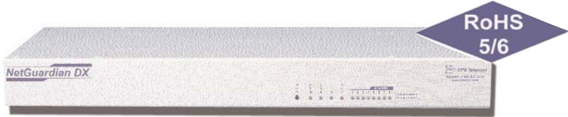
Figure 1 - The NetGuardian Discrete Expansion unit with integrated hub provides an additional 48 alarm points per unit (3 max.), an 8-port 10BaseT hub, and 8 controls to extend capacity of the NetGuardian 832A
